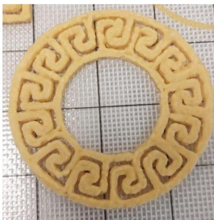
Fig 3: Blast Freeze 3D Printed sample
