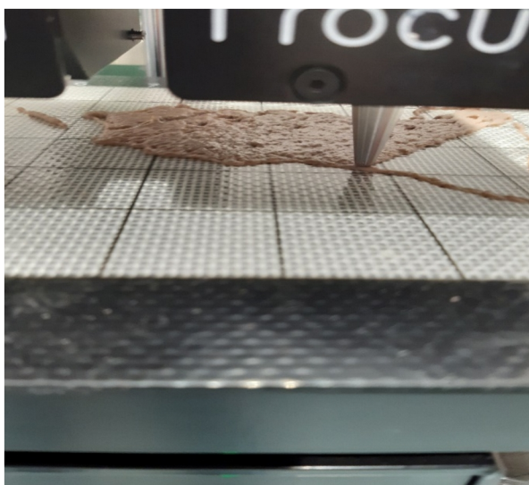
Figure 2. Printing of a steak for those with dysphagia.
