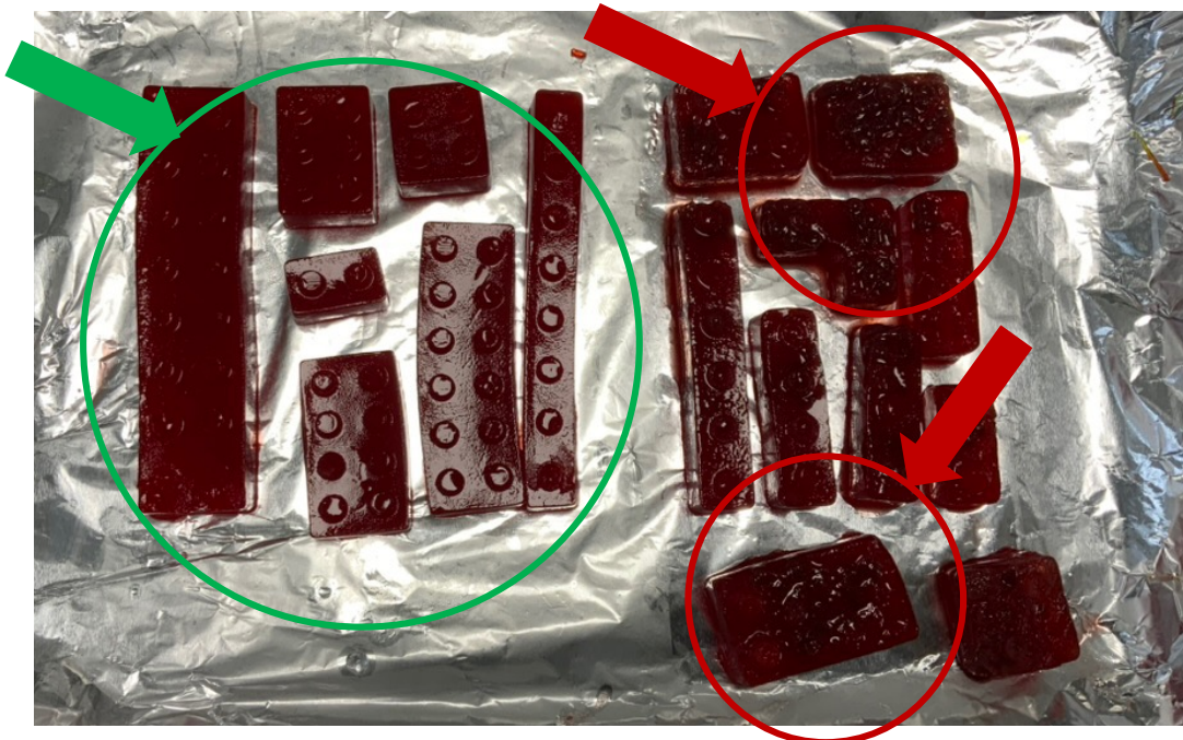
Figure 12. On green, we have the right gelling process, obtaining a very nice and defined shape, on red we have the deformation caused by adding the spheres into the structure.
