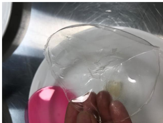
Fig.14. Glycerine + gelatine attempt of edible wrap after 36 h storage in an open locker.
